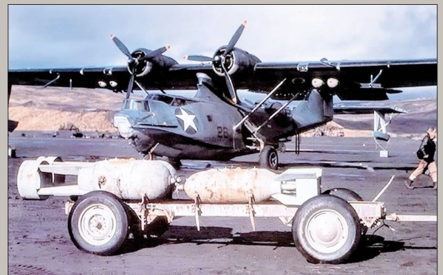
A ‘bombed up’ PBY on the ramp in the Aleutians, 1942-1943. The cart carries 500lb bombs and 100lb depth charges, the aircraft is armed with 500lb bombs as well. Photo – Tumblr.com (continued...)
