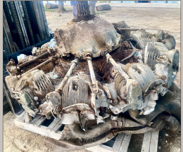
The remains of one of the huge Wright Cyclone R-1820-97 engines that were fitted to the B-17. Once it's been clean up it will go on display at the museum in Luganville. Photo – Bradley Wood.
