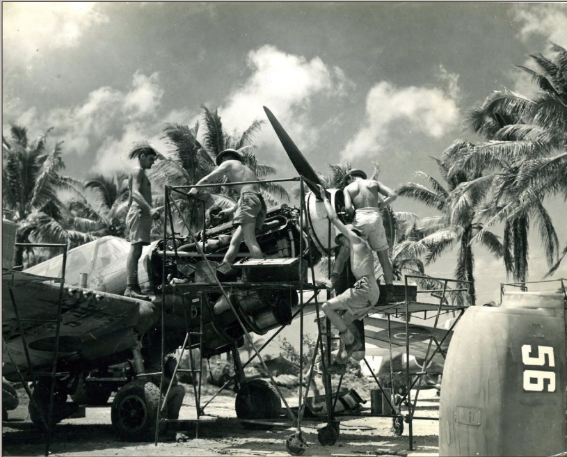
A P-40 of the RNZAF undergoes engine maintenance at Pallikulo Bay Airfield prior to the aircraft heading north to the Solomon Islands frontline oncemore. Photo – John Saunders/Facebook.
