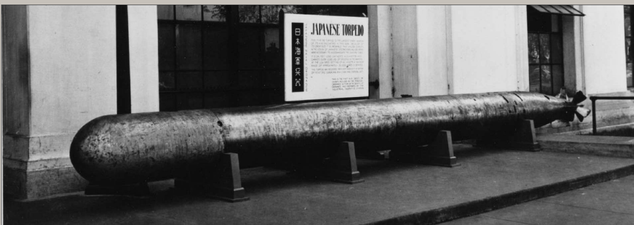
The huge Type 93 "Long Lance" Torpedo that could be fired from great distances from its intended target. Photo – National WWII Museum.
