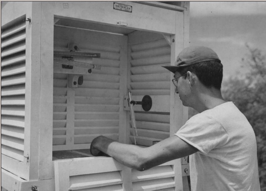
Weatherman S/Sgt John I. Hayes, takes an hourly reading from a psychrometer, an instrument for determining temperature-dewpoint-relative humidity. Photo – US Archives.
