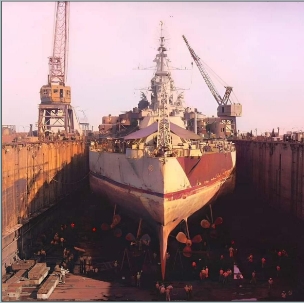
USS West Virginia (BB-48) sits high and dry in ABSD-1 in Pallikulo Bay. The ship was undergoing repairs for damaged propellers after 'touching bottom' following the Battle of Surigao Strait. Photo – Various.
