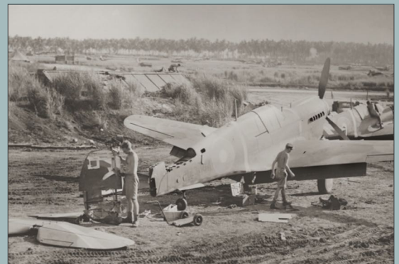
RNZAF P-40 NZ 3064 of 16 Squadron under repair. The tailplane and rudder have been removed, with the rudder showing damage. Another P-40 in front has the engine cowling removed. In the background are other aircraft, some with parts missing. From Geoff Fiskin's personal collection. Photo – Masterton District Library.
