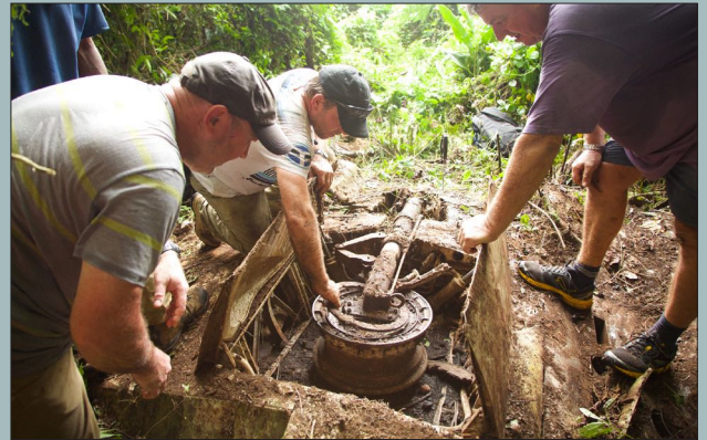
The landing gear of a crashed RNZAF Corsair is inspected by a team from the South Pacific WWII Museum. Photo – Karl von Moller.
