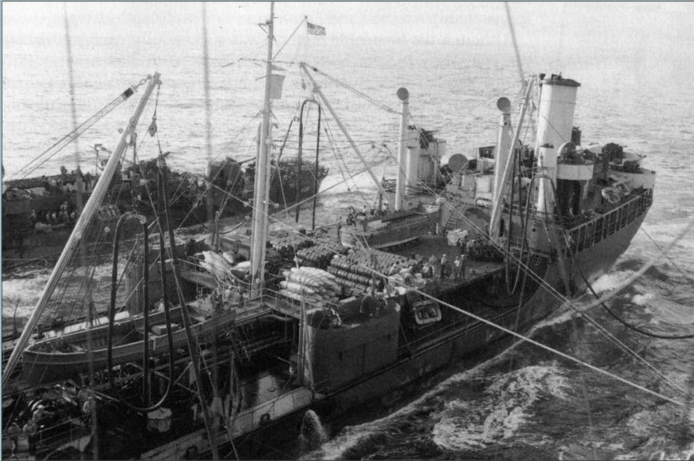
By the end of the war, oilers were routinely transferring stores and munitions while conducting fueling at sea. Extra belly tanks for aircraft and containers of ammunition were often stowed on the open spar deck, as can be seen in this photo. Photo – US Archives.
