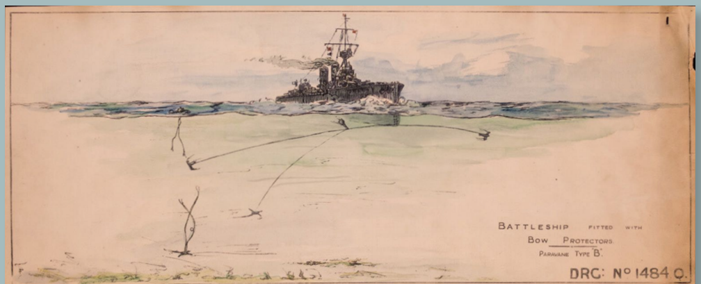
Battleship, with bow protectors: paravane type B. c1916 – Institution of Mechanical Engineers.
