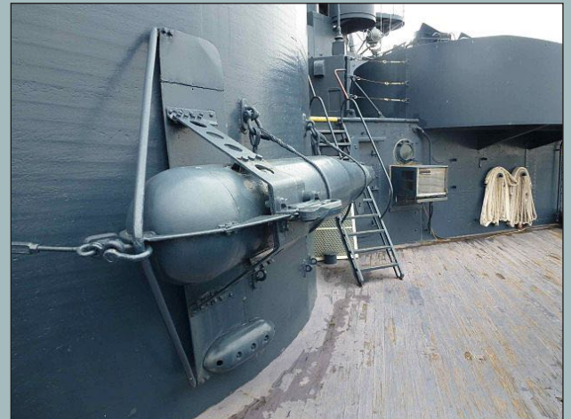
A paravane in its transport position, mounted to the superstructure of the USS Texas in San Jacinto State Park, near Houston Texas. Photo – Wikipedia.
