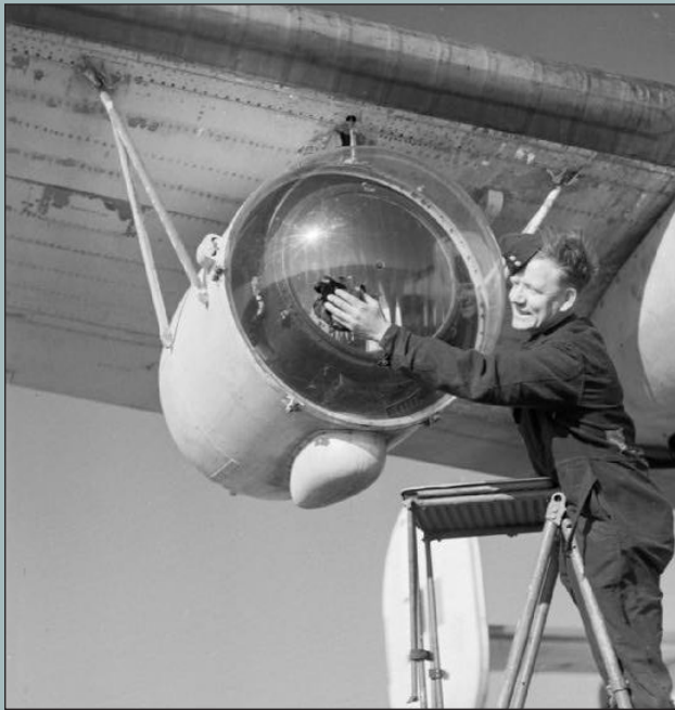
A Leigh Light fitted under the wing of a Consolidated Liberator aircraft of the Royal Air Force Coastal Command, 26 February 1944. The 22 million candlepower light was also used by the US Navy in the Pacific. Photo – Imperial War Museum.
