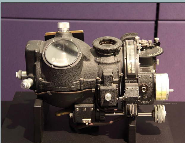
The Norden bombsight at the Computer History Museum in Mountain View, California. This example is only the bombsight itself; it does not include the associated autopilot that would normally connect to it on the bottom. Photo – Allan J Cronin.
