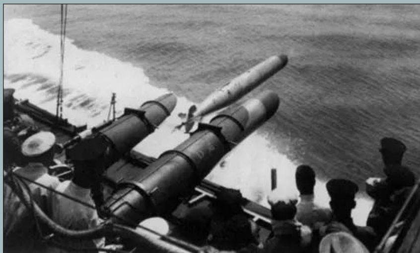
A Japanese Type 93 'Long Lance' torpedo being launched. Photo - Tides of History
