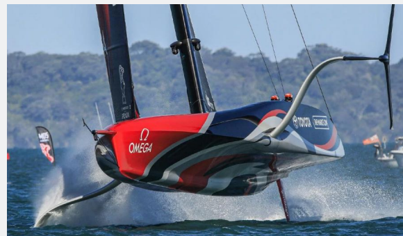
Emirates Team New Zealand America's Cup boat - a high performance fully foiling monohull racing yacht. Pic - Emirates Team New Zealand.
