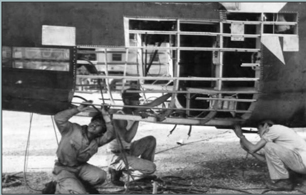
29th Air Service Group ground crew repair the tail section of a Consolidated Liberator bomber. Photo US Archives.
