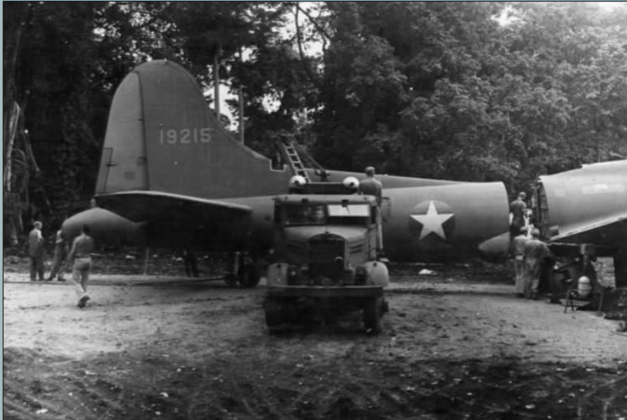
A B-17 Flying Fortress is given a new tail by crews of the 29th Air Service Group on Santo. Photo US Archives.
