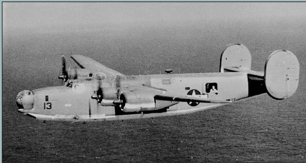
PB4Y-1P photo reconnaissance aircraft of VD-1 near Guadalcanal, 1944. Cameras are on the bottom of the aircraft and in the tail behind the star. Photo pacificairlifter.com/vpnavy.org
