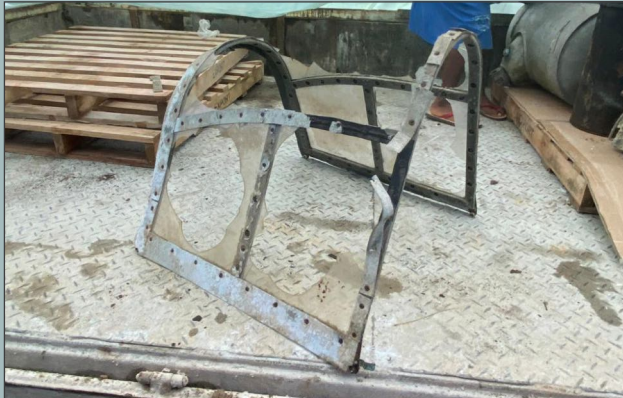
The fantastic SBD Dauntless canopy still in great condition – apart from the odd broken piece of plexiglass.
