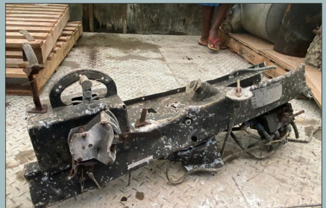
One of the more exciting pieces donated to us in this left side panel from the cockpit of an F4U Corsair fighter aircraft.
