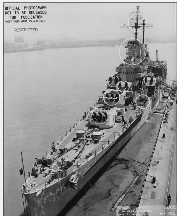
Denver at the Mare Island Navy Yard following her overhaul. Circles mark recent alterations to the ship, including a new radar. 1 May 1944. Photo Naval History and Heritage Command.
