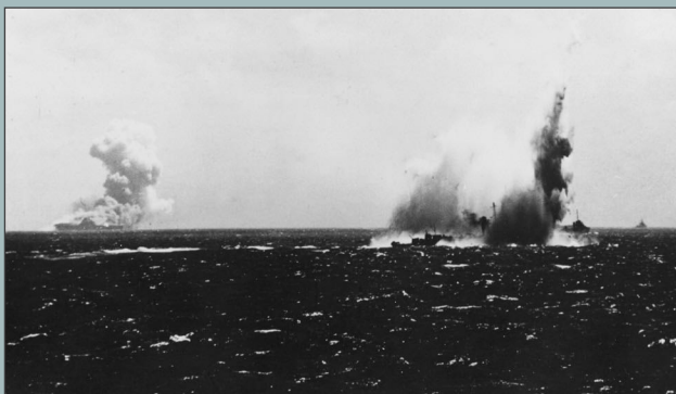
The USS O'Brien is torpedoed by the Japanese submarine I-19 during the Guadalcanal Campaign, on 15 September 1942. The aircraft carrier USS Wasp (CV-7), torpedoed a few minutes earlier, is burning in the left distance. O'Brien was hit in the extreme bow, but "whipping" from the torpedo explosion caused serious damage to her hull amidships. Photo US Archives.
