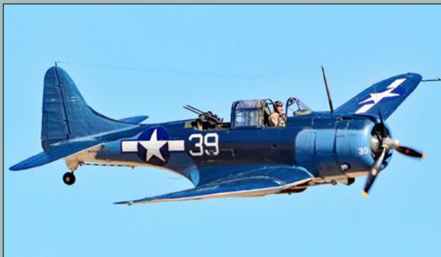
A restored SBD-5 Dauntless, featuring the twin Browning machine guns. Photo Planes of Fame Air Museum/Wikipedia.
