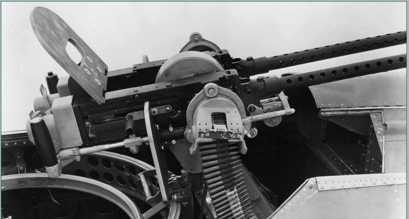
A close up detail photo of the Browning machine guns showing the thick steel bullet-proof screen to protect the rear gunner.
