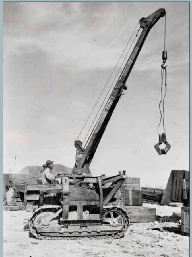
A version of the TD-9 with similar features to the South Santo TD-9. Both the US Army and the USMC used a version of this tractor crane based on the IH T-9 gas or TD-9 diesel crawler. The USMC version is shown here. Both featured a 2-ton crane from Trackson. The US Army version was called the tractor crane 2-ton M5 and featured a 334.5-cubic-inch, 46-belt-horsepower gasoline engine (52 horsepower on the flywheel). The USMC version had a diesel engine that displaced 334.5 cubic inches and made 44 belt horsepower. Photo Wisconsin Historical Society
