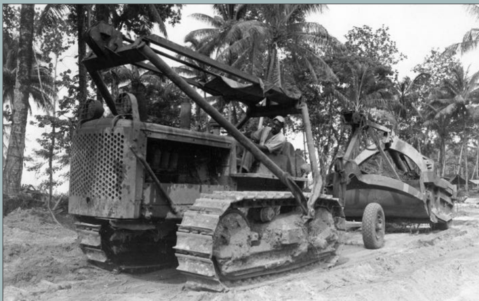
A US Navy Seabee crawler pulling a modified 'Carry-All' minus a blade which would have made it a bulldozer..
