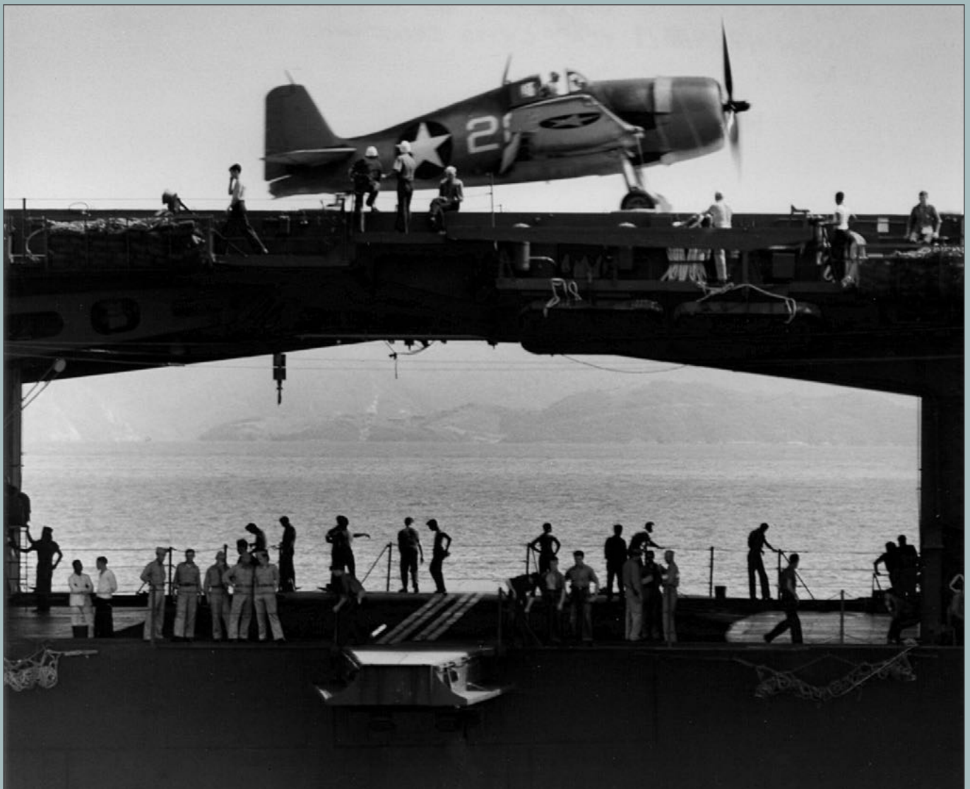
An F6F from VF-1 can be seen on the main deck of the USS Yorktown (CV-10). While below, the ship's hangar catapult is clearly visible. Photo US Navy.
