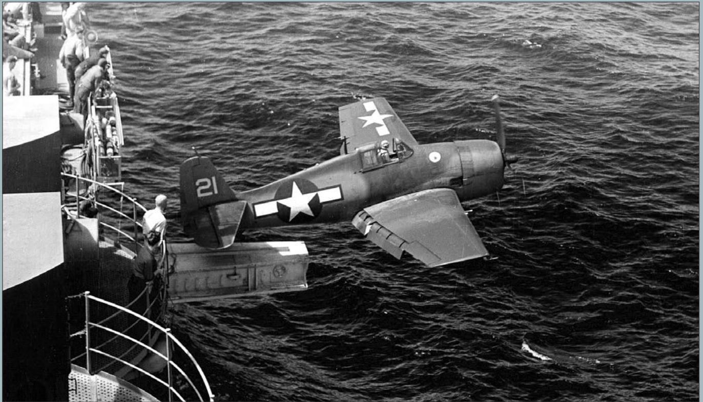
An F6F Hellcat launches off USS Hornet's hangar catapult, Photo US Navy.
