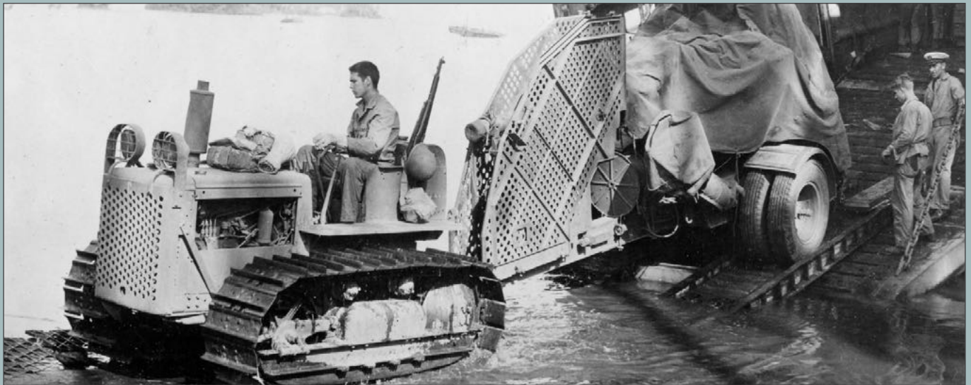
A Caterpillar D4 is seen pulling a load off of a Landing Craft, Medium, during a practice landing in the Pacific Theatre. Photo usautoindustryworldwartwo.com
