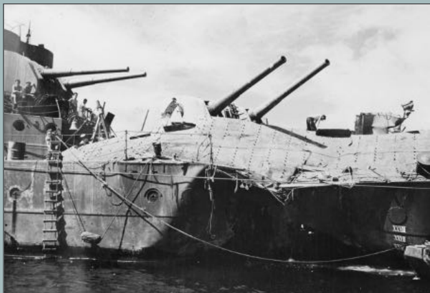
Photographed from off the port side showing the ship's badly distorted stern, after Hobart arrived in Espiritu Santo. AWM photo.
