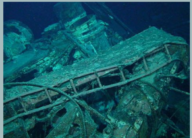
The wreck of the Centaur discovered in 2009 shows the collapsed foremast due to implosion as a result of the rapid sinking of the ship Source: David L Mearns, Search Director, The Finding Centaur Project. qldwarmemorials.com.au
