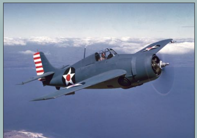
A U.S. Navy Grumman F4F-3 Wildcat in non-specular blue-grey over light-grey scheme in early 1942. Photo Wikipedia.
