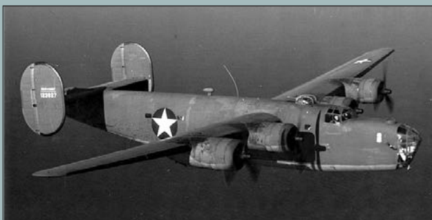
A U.S. Navy Consolidated PB4Y-1 Liberator in flight, in 1943. This aircraft was a USAAF Consolidated B-24D-7-CO transferred to the U.S. Navy. It still wears the standard USAAF camouflage. Photo Wikipedia.
