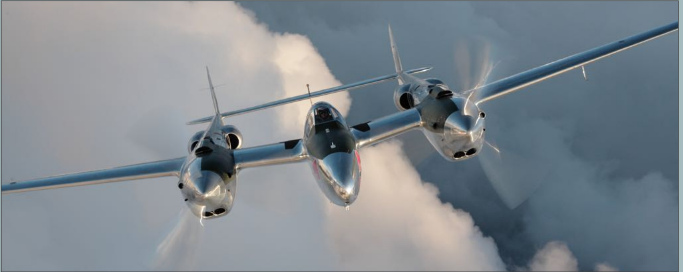
The only P-38 in Europe, is owned by the Flying Bulls in Austria. This stunning example took four years to restore and its aluminium skin polished to a mirror-like finish. Picture flyingbulls.at
