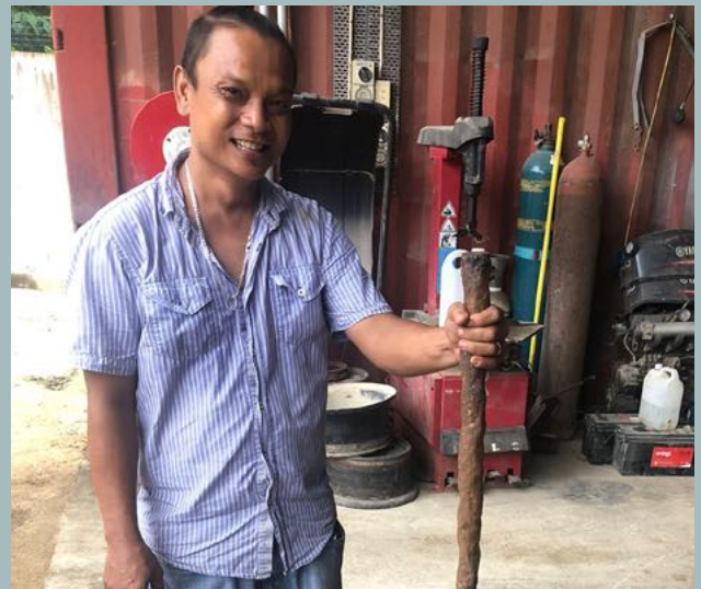
Rommel Tugalon is holding the badly corroded steel rod that holds the whistle together. Yves turned and threaded a new one to fit the whistle.
