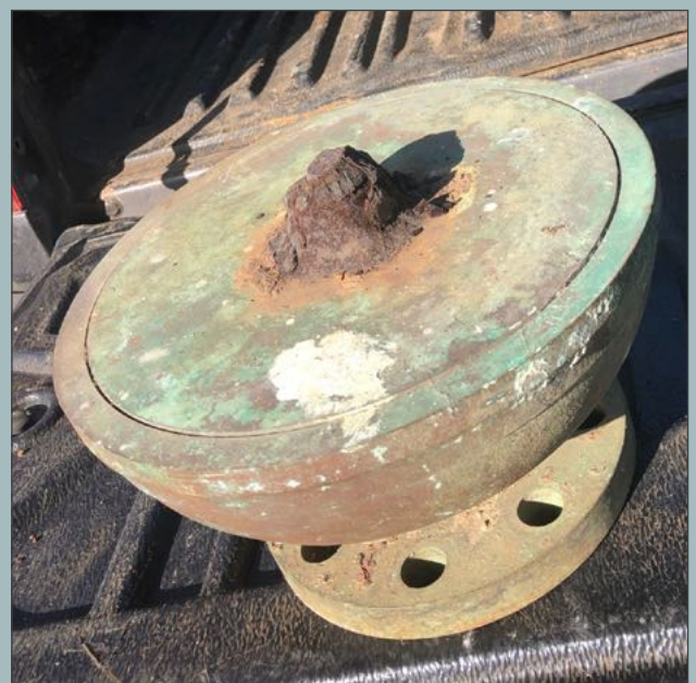
The heavy brass base of the whistle. Compressed air gets forced through the base, exiting via the circular gap around the top.
