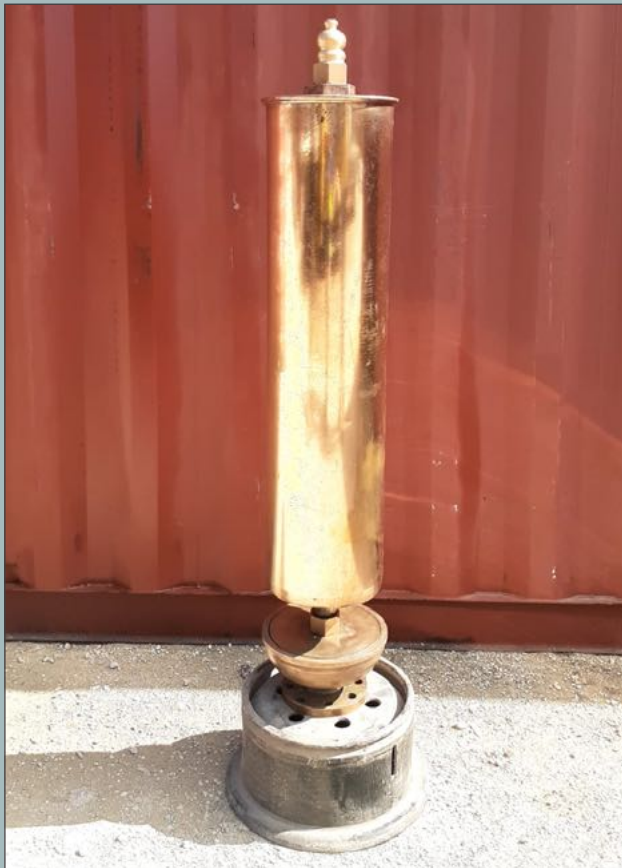
The completed Coolidge whistle ready for testing and tuning.
