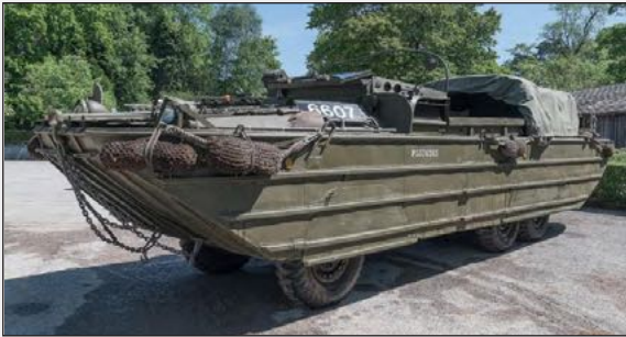
A US Army DUKW or 'duck'. One of the American trucks that "could go on both the land and sea." Photo keymilitary.com
