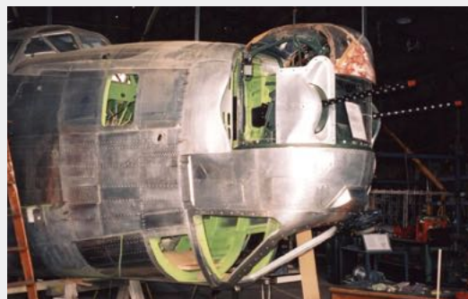
The B-24's nose turret under restoration at Werribee. Photo: B-24 Liberator Restoration Australia.
